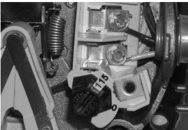
Figure 4: Motor Set for 115 Volt Operation
