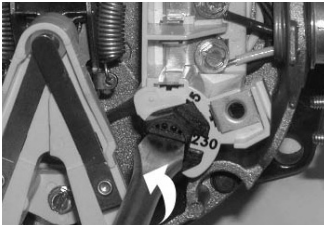
Figure 3: Changing the Voltage Setting
