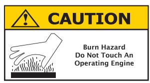
Engines can operate at high temperatures. To avoid burns when servicing pump, allow it to cool for 60 minutes after shutdown before handling.
