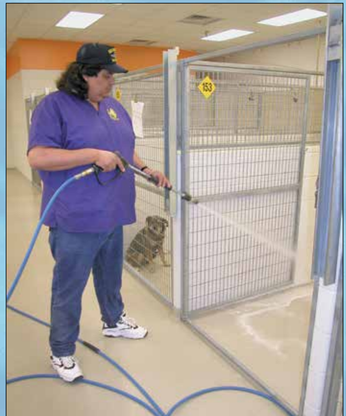
“On-Demand” soap injection at the wand provides for highly effective and fast coverage of all kennel walls and floors.
