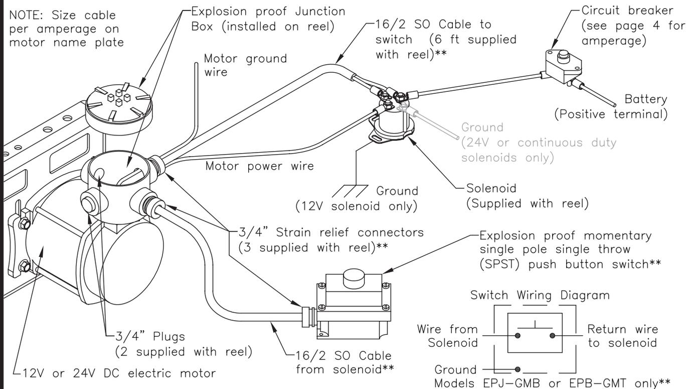
**\*\* NOTE-**If reel is equipped with Hannay Guidemaster (model prefix EPB-GMB or EPB-GMT), then switch and cord are replaced with Guidemaster switch and accompanying mounting hardware. Additionally, only 2 strain relief connectors are provided. See note on wiring diagram for installing Guidemaster switch.
